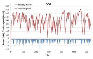
Fig. 4. Braking energy and vehicle speed during SS1
