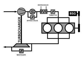
Fig. 2. Diagram of the analyzed 48 V hybrid system
