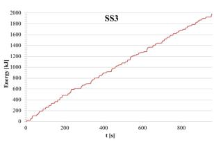
Fig. 9. Braking energy in SS3
