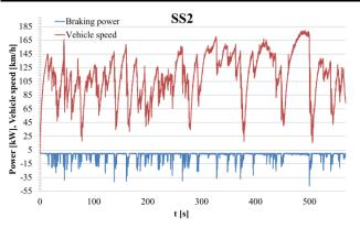
Fig. 5. Braking energy and vehicle speed during SS2
