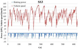
Fig. 6. Braking energy and vehicle speed during SS3
