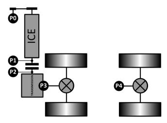
Fig. 1. Possible variants of the 48 V hybrid drivetrains in the car
